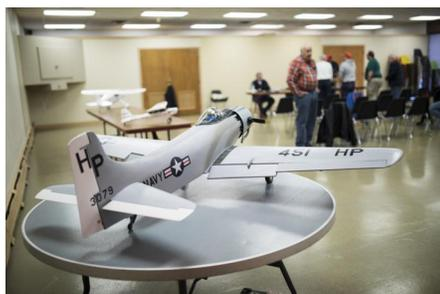
Gerardo of course brought in a large plane. It's an sbach 342 107" wingspan. It should take a 100cc engine but it has a 120 twin DLE. Prop is a 29x9 cf prop. 8 HV servos running 6V on a 9ch JR dsm2 receiver. 1 servo per channel with slave channels for the servos that are duplicated. Like the ailerons that have 2 servos. Onboard is a power distribution box that guarantees the voltage at all times. It has 4 satellite receivers and the plane weighs about 35 lbs.
