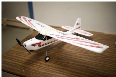
Hal and Gary brought in a SkyRaider that's a Charlie Bower (sp?) design. It was designed as a "Ready to Cover". Hal had some issues trying to Monokote the Fiberglass and it didn't work out well. Fabrikote seemed to do the trick. Then Monokote on top. These steps saved him from having to paint the entire plane. It weighs about 7.5-8 lbs. 140 Engine. All the numbers are monokote. Hasn't flown yet.
